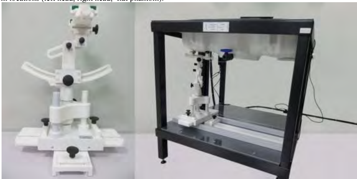
Device holder supplied by SATIMO
