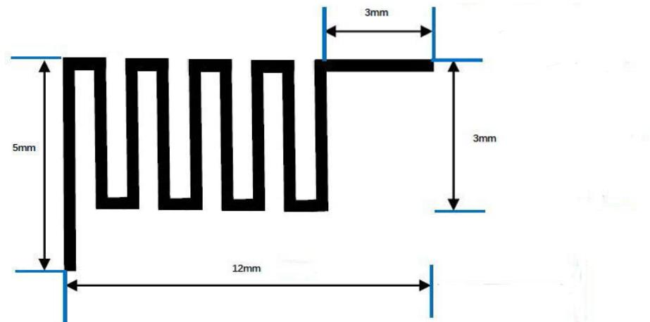
Since there is no ground plane beneath the antenna, PCB thickness will have little effect on the performance. The results presented in this design note are based on an antenna implemented on a PCB with 1 mm thickness.
