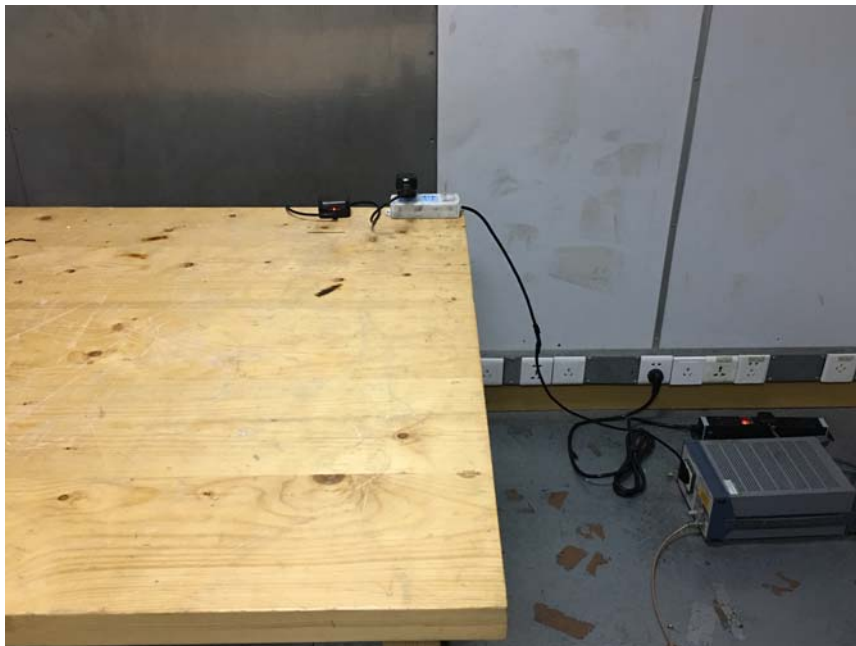
Photograph of set-up for conducted Emission
