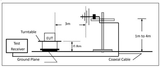
(c) For radiated emissions above 1000MHz
