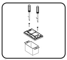
If you want to install on the junction box, use the screw in the package and a cross screwdriver to lock the device on the junction box
