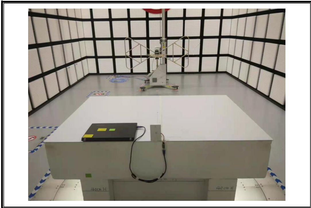
RADIATED RF MEASUREMENT SETUP (30MHz ~ 1 GHz)
