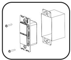
Install the back housing(s) of the wall dimmer(s) into the wall box.
