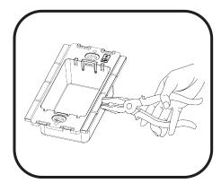
For proper installation into a dual gang junction box, the tabs between adjacent back housings must be removed. Carefully observe the correct orientation (the UP arrow should be in the upper right corner on each back housing). After double checking the product orientation, break off the necessary tabs using pliers.
