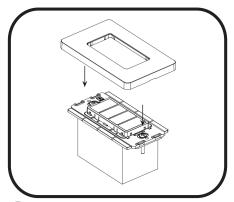
Install the faceplate onto the device. Note: Device supports the use of other standard faceplates on the market.
