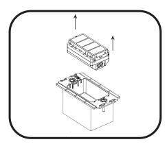
Remove the device from the back housing.
