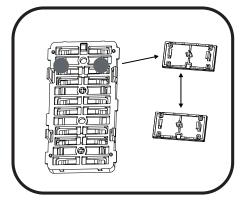
Remove the individual buttons and replace with the new set of buttons.
