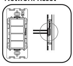
To reset the network of the device, remove the faceplate from the device. Then press and hold the reset button for 5 seconds. Install the faceplate back onto the device. Press either dimming up or down button to enter the pairing mode to join the device to a network.
