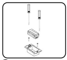
Use a standard screwdriver to remove the devices from the back housing
