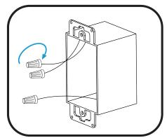
Reconnect wires (previously connected to wall switch) with wire nuts.
