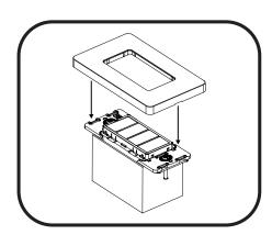
Install the faceplate onto the device. The device will rejoin its network automatically.
