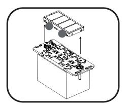
Squeeze the clip on the side of the button to take off the button module from the devices
