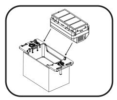
Remove the device from the back housing.
