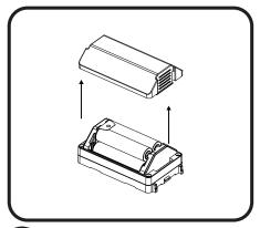
Separate the battery cover from the device. Pull the plastic insulation strip out of the battery compartment. Put the battery cover back on the device.
