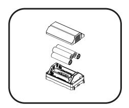
Separate the battery cover from the device. Replace the batteries with AAA batteries. All batteries need to be replaced at the same time.
