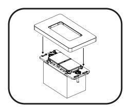
Install the faceplate onto the device. The device will rejoin its network automatically.
