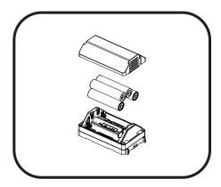
Separate the battery cover from the device. Replace the batteries with AAA batteries. All batteries need to be replaced at the same time.
