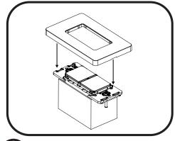
Install the faceplate onto the device. Note: Device supports the use of other standard faceplates on the market.
