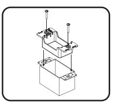
Insert the back housing piece into the junction box and secure with two screws.
