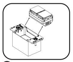
Install the main body of the device into the back housing.
