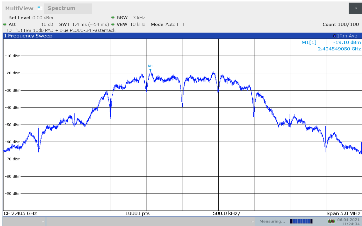
Figure 8.7-1: Power spectral density of digital transmission system, 2405 MHz
