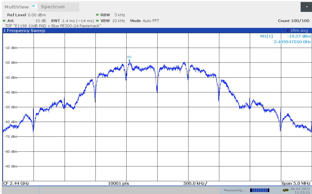
Figure 8.7-2: Power spectral density of digital transmission system, 2440 MHz
