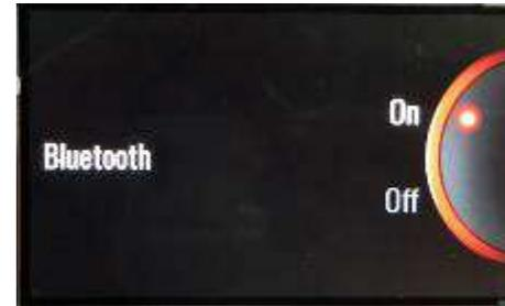
Short press of UP SW to move the selection to ON then short press of Select SW to confirm.
