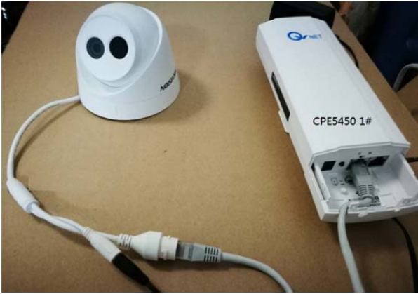
2-1-2 Use Ethernet cable to connect LAN port of CPE5450 1# to POE port of power adapter
