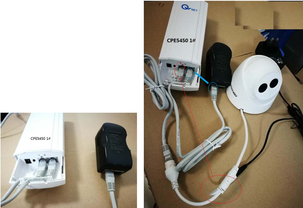
2-1-2 Use Ethernet cable to connect LAN port of CPE5450 1# to POE port of power adapter
