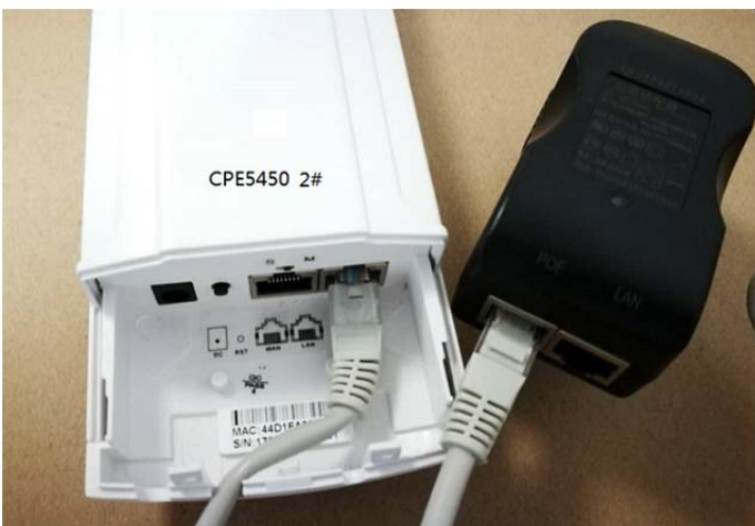
2-1-3 Use Ethernet cable to connect LAN port of CPE5450 2# to POE port of power adapter
