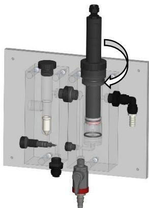
Lock the tightening nut until the O-ring seals.
