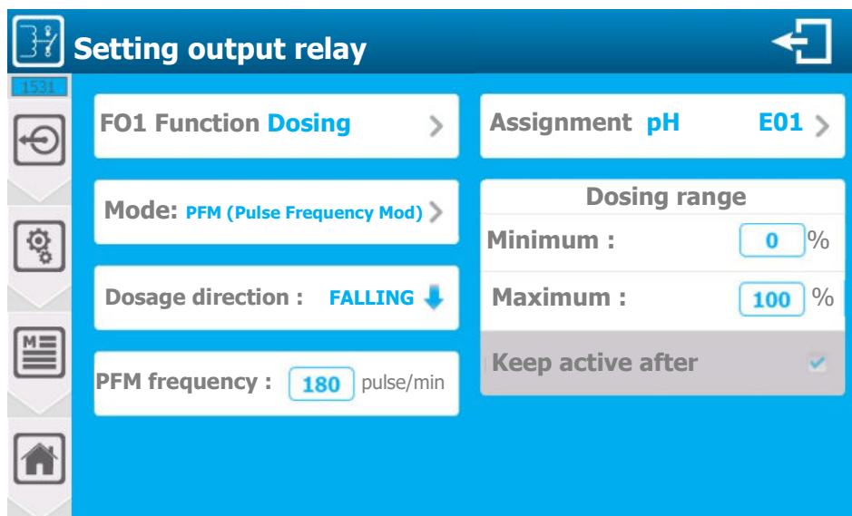
c) Relay outputs in PFM (Pulse Frequency Modulation) dosing mode [1531]
