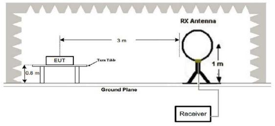
(2) Radiated Emission Test-Up Frequency 30MHz~1GHz
