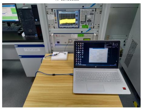
Conducted Emission For AC Mains Power Ports
