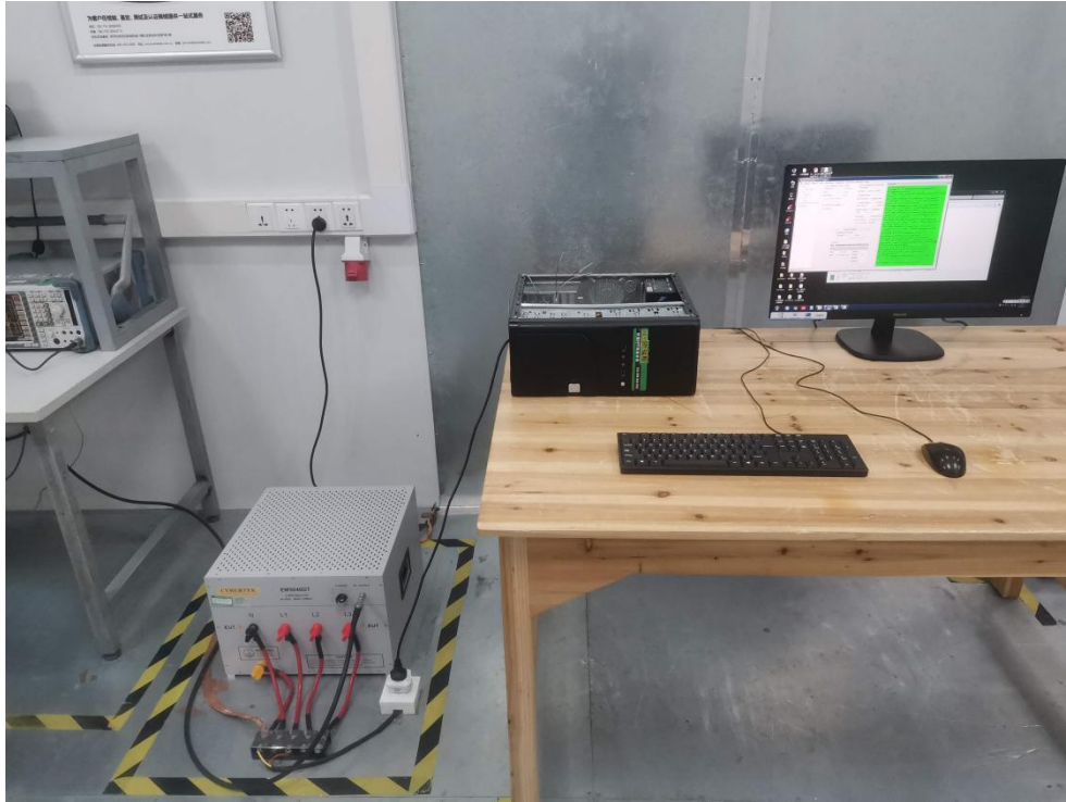
Photo of Power Line Conducted Emission Test
