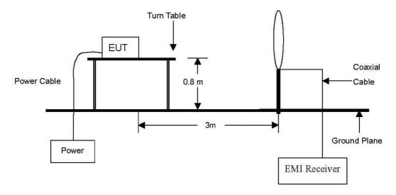
The diagram below shows the test setup that is utilized to make the measurements for emission from 30  $\,\mathrm{Mz}$  to 1  $\,\mathrm{Gz}$ .
