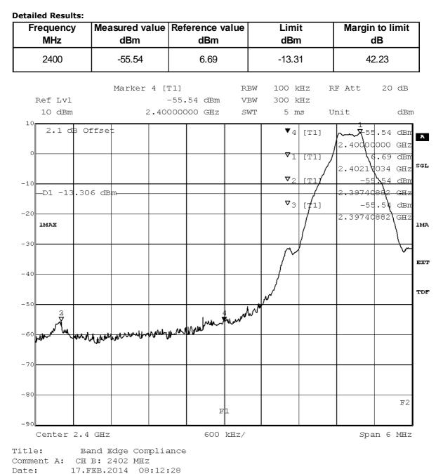
Test: 15c.6; Frequency = 2402, Mode = BT transmit using 2 Mbps with PI/4 DQPSK modulation, Method = conducted
