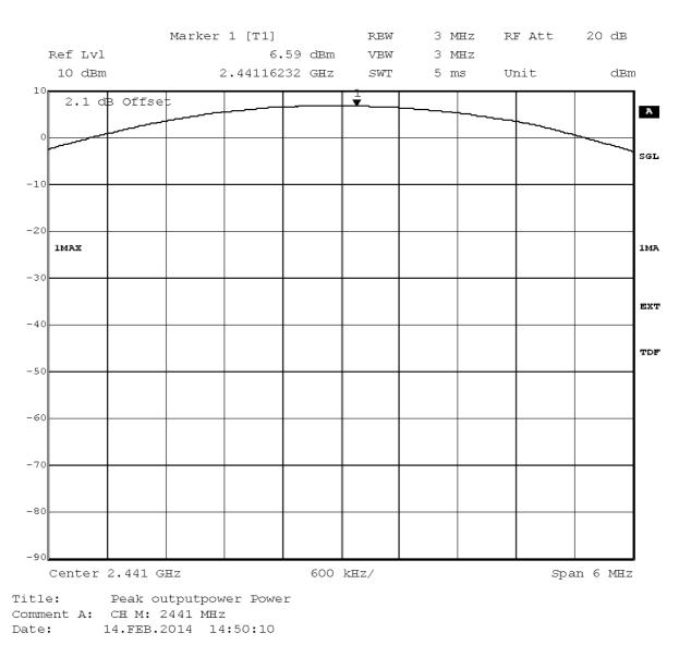
Test: 15c.4; Frequency = 2441, Mode = BT transmit using 2 Mbps with PI/4 DQPSK modulation
