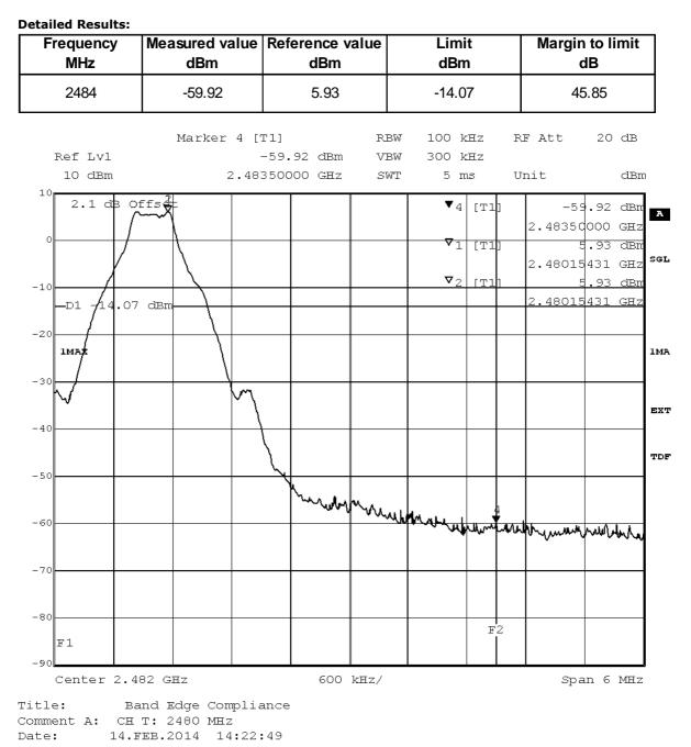
Test: 15c.6; Frequency = 2480, Mode = BT transmit using 1 Mbps with GFSK modulation, Method = radiated
