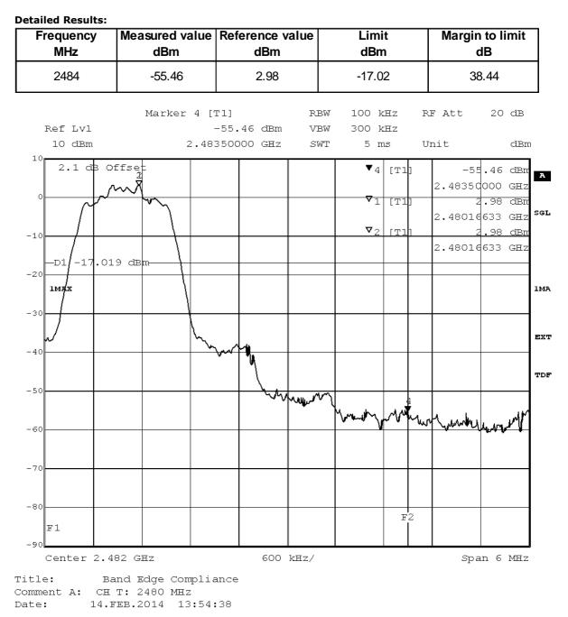
Test: 15c.6; Frequency = 2480, Mode = BT transmit using 3 Mbps with 8DPSK modulation, Method = radiated
