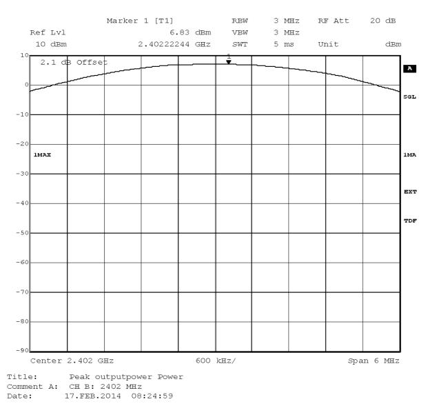
Test: 15c.4; Frequency = 2402, Mode = BT transmit using 2 Mbps with PI/4 DQPSK modulation
