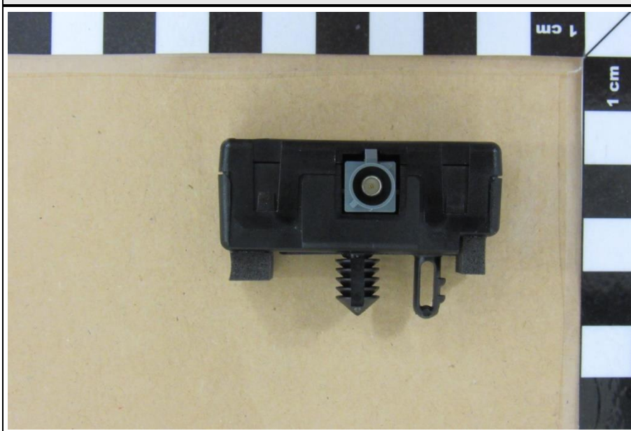
Wifi antenna 5B4.035.510 side view
