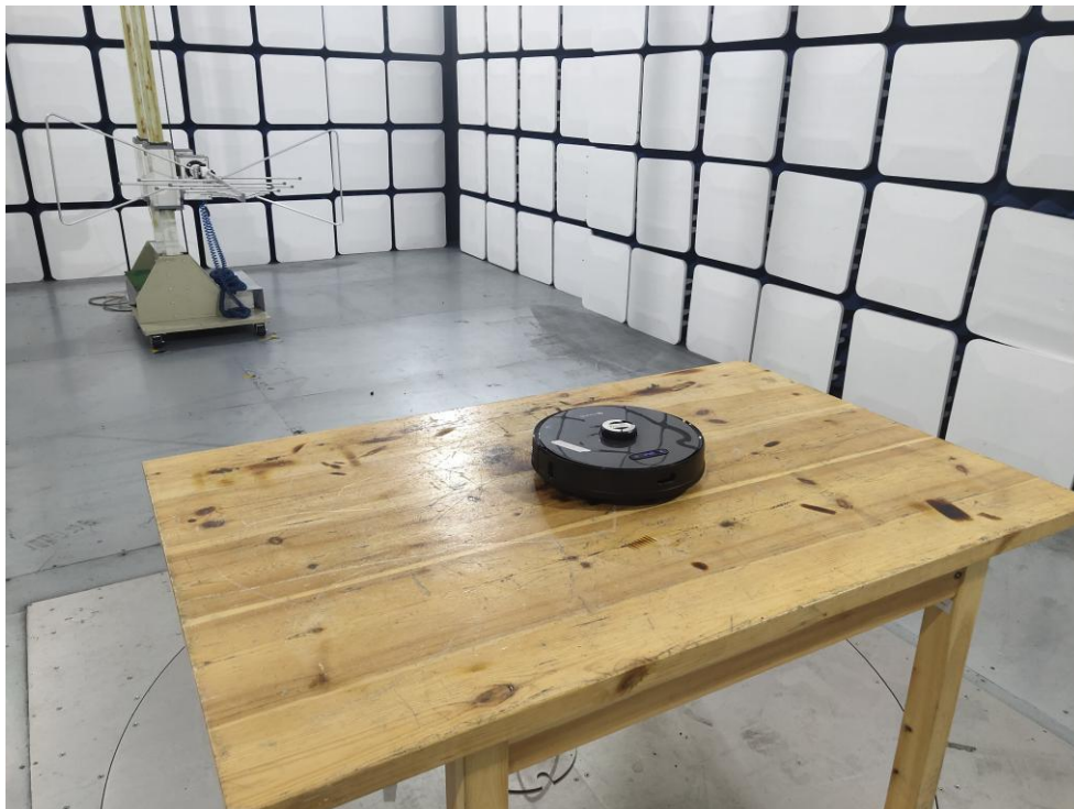
Photo of Radiation Emission Test
