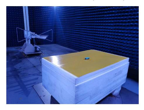
**Radiated Emissions Test View (Above 1GHz)**
