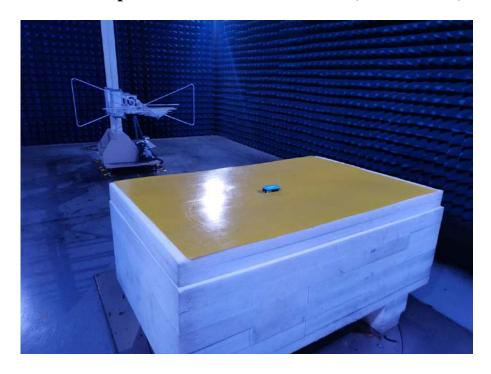
**Radiated Spurious Emissions Test View (Above 1GHz)**
