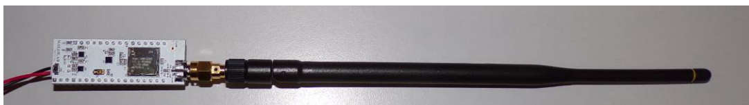
Test board + antenna #2 (1/2 Wave Antenna with maximum gain 2.2 dBi)
