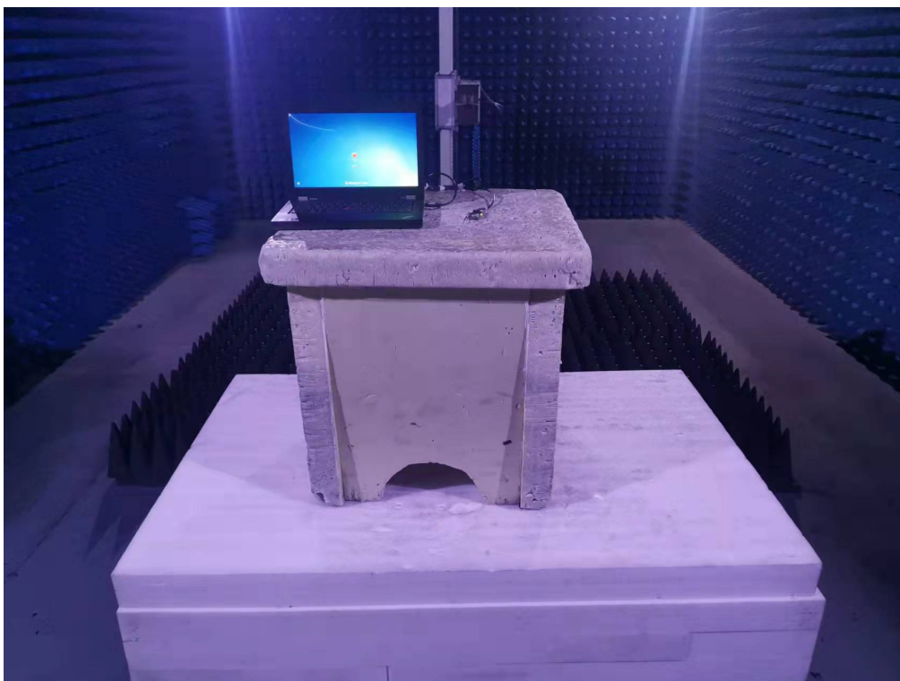
Photo of Radiated Emission Measurement (Above 1G)
