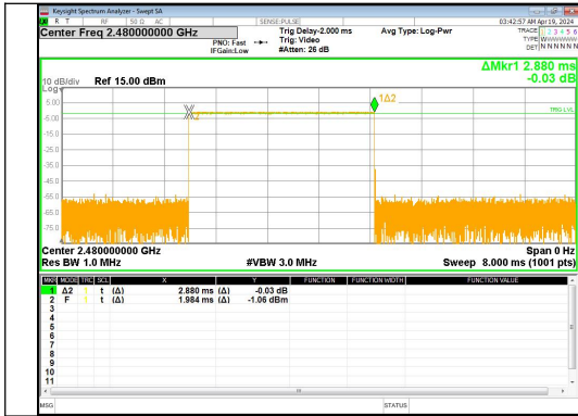
Pulse Width GFSK_DH5
