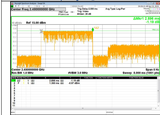
Pulse Width 8DPSK_3-DH5
