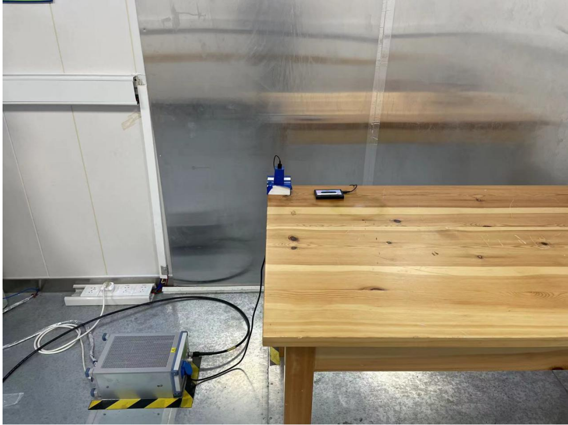
Conducted emission test setup
