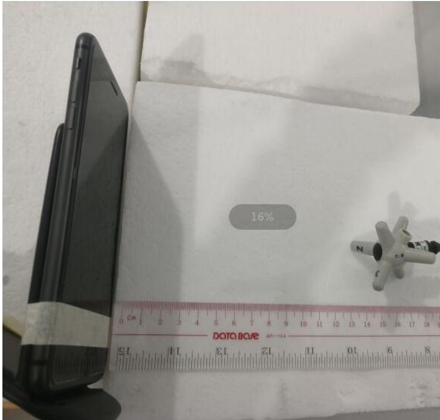
E-field Test Setup Photo Positon E(15mm)
