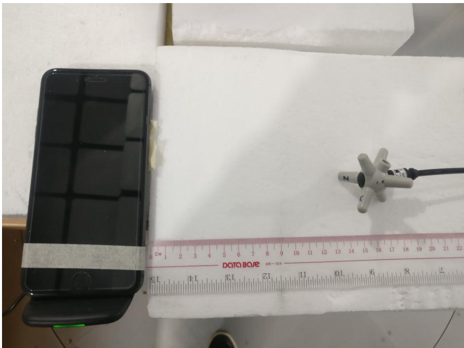
E-field Test Setup Photo Positon D(15mm)
