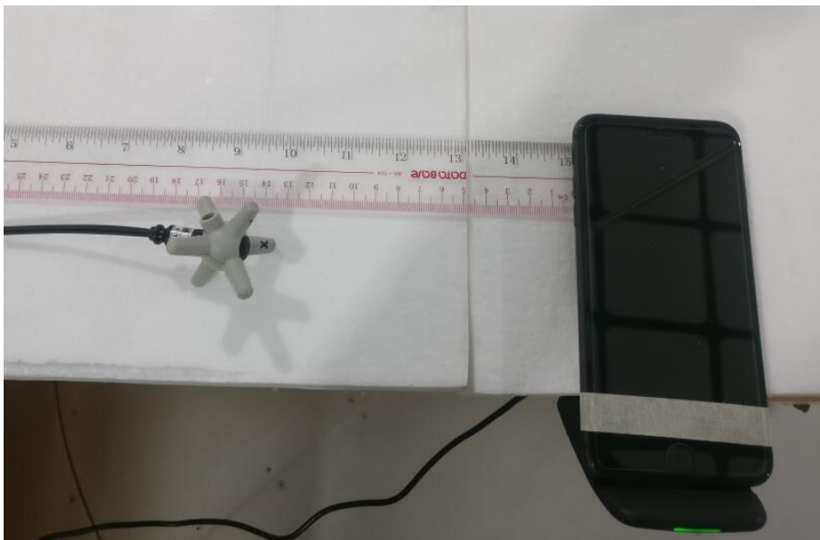
E-field Test Setup Photo Positon B(15mm)
