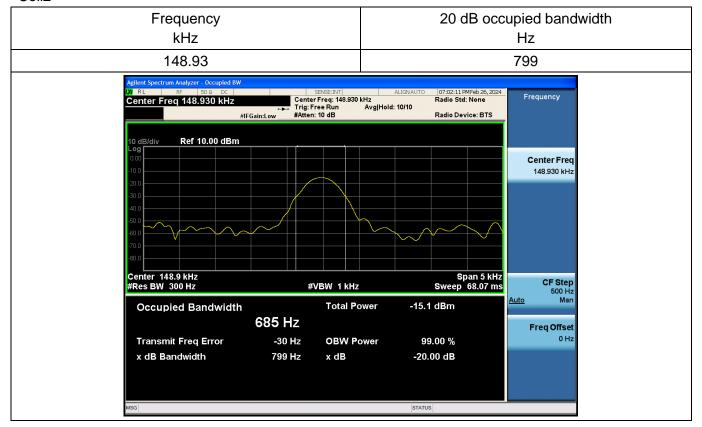
**Note:** Because the measured signal is CW-like, adjusting the RBW per C63.10 would not be practical since measurement bandwidth will always follow the RBW. The RBW is set to 300 Hz to perform the occupied bandwidth test.
