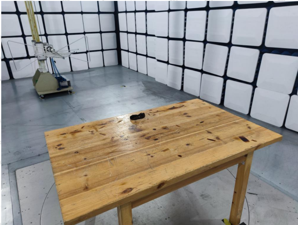
Photo of Radiation Emission Test
