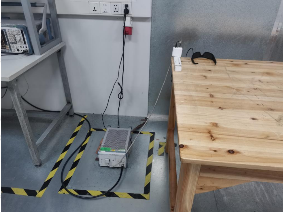
Photo of Conducted Emission Measurement
