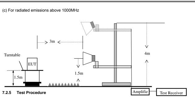
The test site semi-anechoic chamber has met the requirement of NSA tolerance 4 dB according to the standards: ANSI C63.10-2013. The test distance is 3m. The setup is according to the requirements in Section 13.1.4.1 of ANSI C63.10-2013 and CAN/CSA-CEI/IEC CISPR 22.
