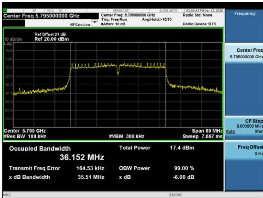
**6 dB Bandwidth:****802.11ac-VHT80 CH5775MHz**
