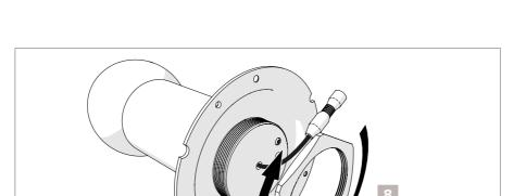
8. Fasten the lamp holder by turning the lamp lid on to the LED light.
