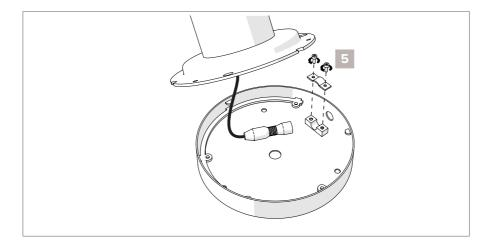
5. Loosen the Allen screws of the strain relief.
