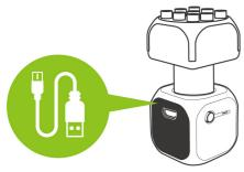
1 After connecting the USB cable to the USB charging adapter, plug them into the connection jack on the back of the module
