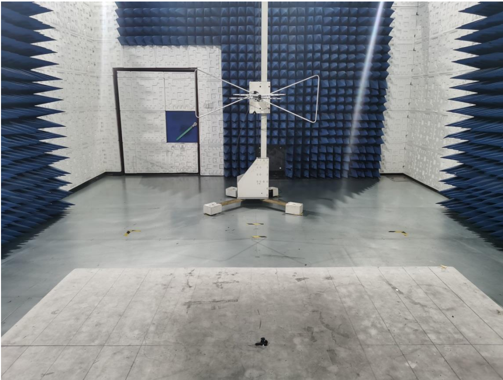
RADIATED EMISSION TEST SETUP ABOVE 1GHz
