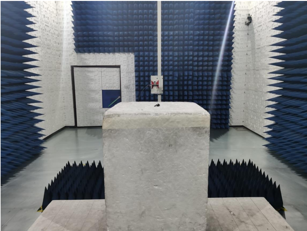
RADIATED EMISSION TEST SETUP ABOVE 1GHz
