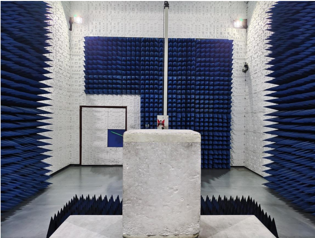
RADIATED EMISSION TEST SETUP ABOVE 1GHz
