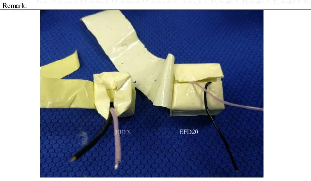
Details of: Transformers view of LED driver for both models Remark:
