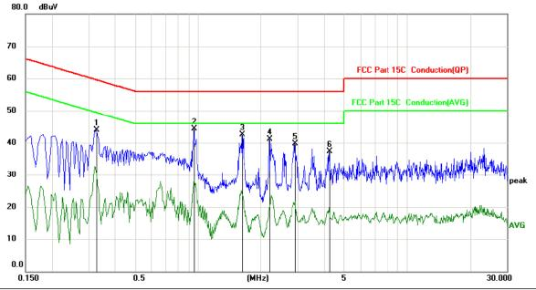
Limit: FCC Part 15C Conduction(QP)
