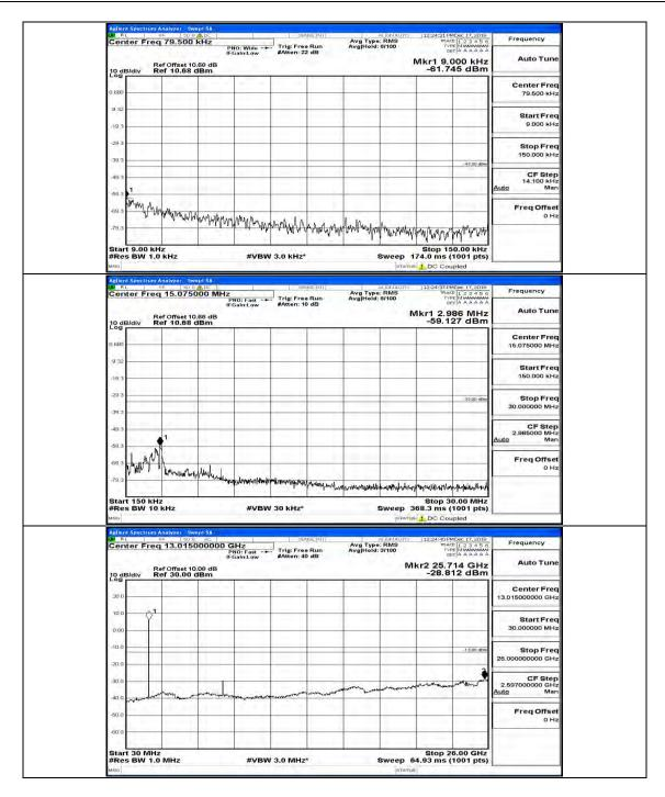
Channel Bandwidth: 10 MHz\_MCH\_16QAM\_1RB#0
