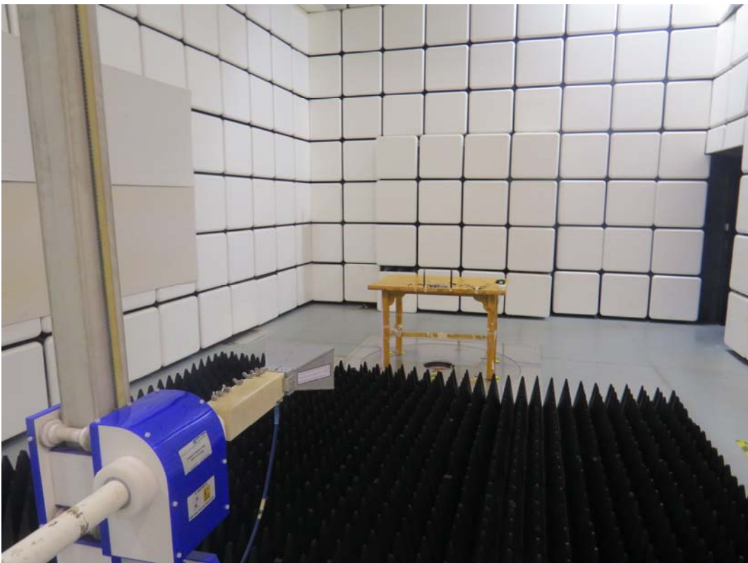
Picture 2: Radiated Spurious Emissions Test setup
