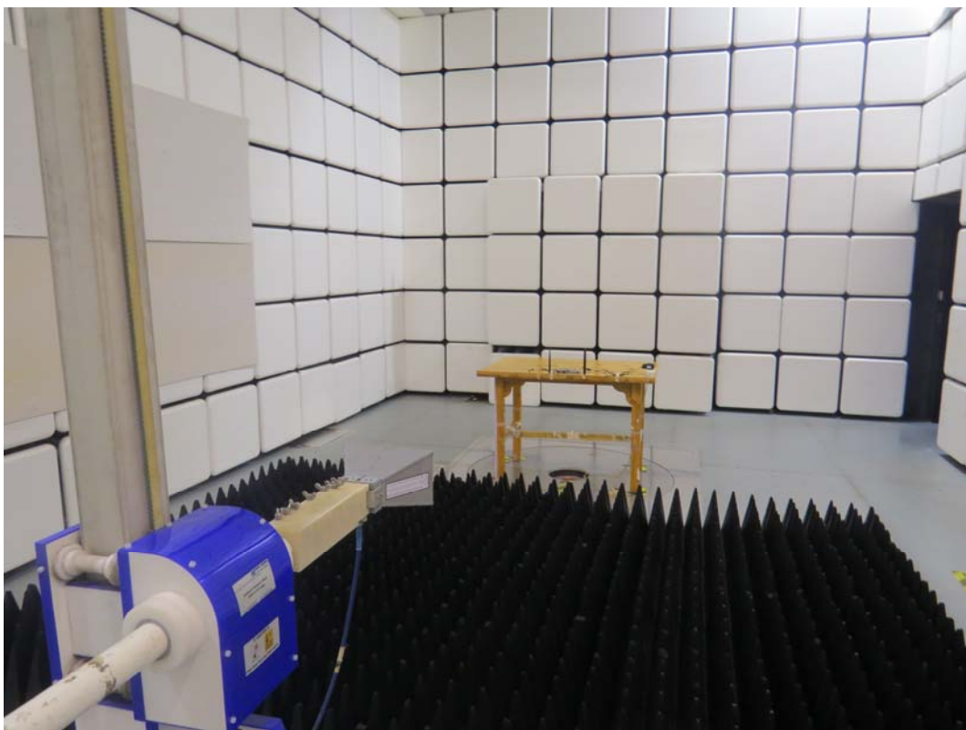
Picture 2: Radiated Spurious Emissions Test setup
