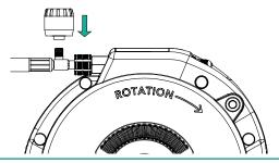
▲ WARNING: A contaminated, corroded, or damaged valve stem or sensor seal may cause a poor seal between the sensor and valve stem resulting in a tire leak.
