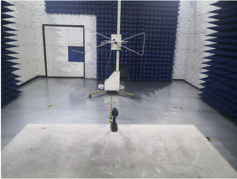
RADIATED EMISSION TEST SETUP ABOVE 1GHz
