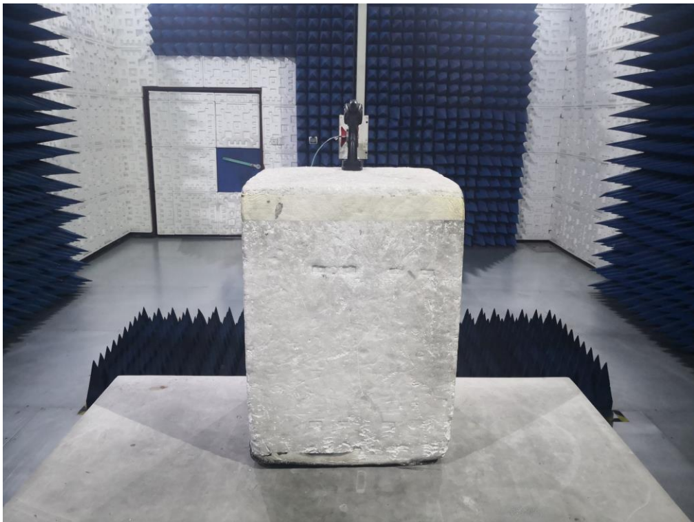
RADIATED EMISSION TEST SETUP ABOVE 1GHz
