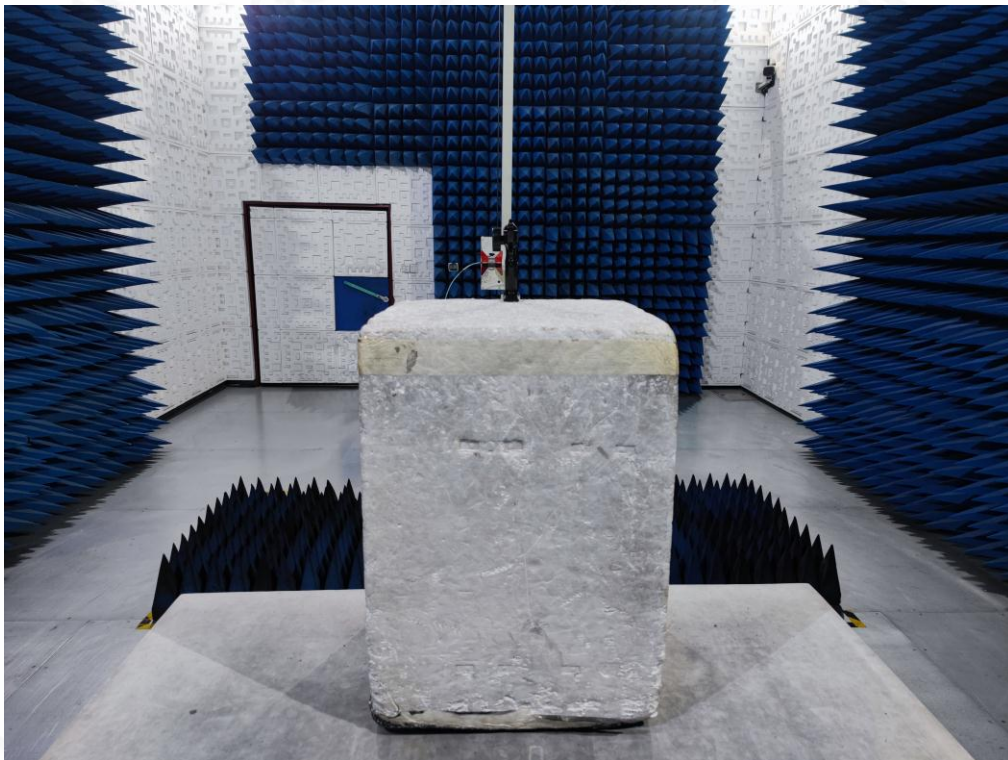
RADIATED EMISSION TEST SETUP ABOVE 1GHZ
