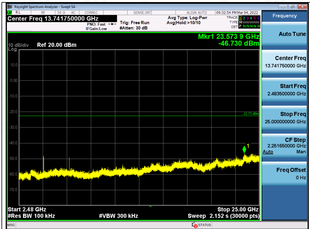
Test_Graph_GFSK_ANT1_2405_Higher Band Emissions
