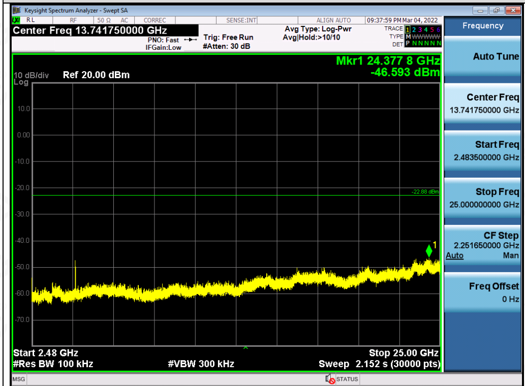
Test_Graph_GFSK_ANT1_2445_Higher Band Emissions
