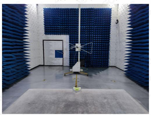
RADIATED EMISSION TEST SETUP ABOVE 1GHz
