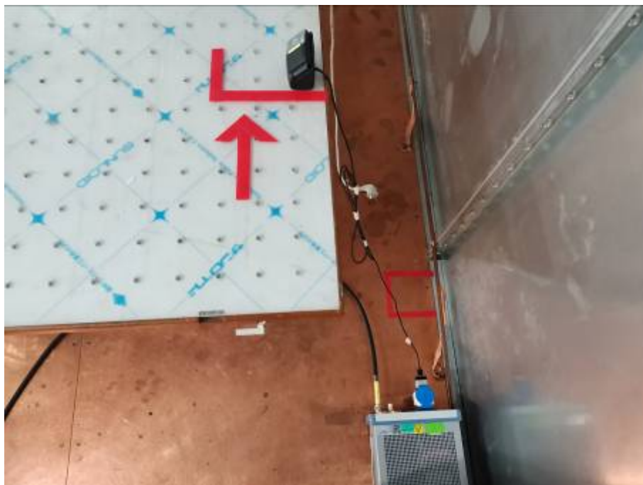
Conducted Emissions Test Setup (with charger)
