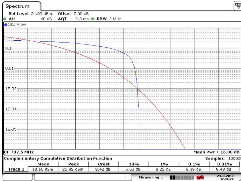
Peak-Average Ratio Plot(5MHz BW,QPSK,Band 12-mid Channel)
