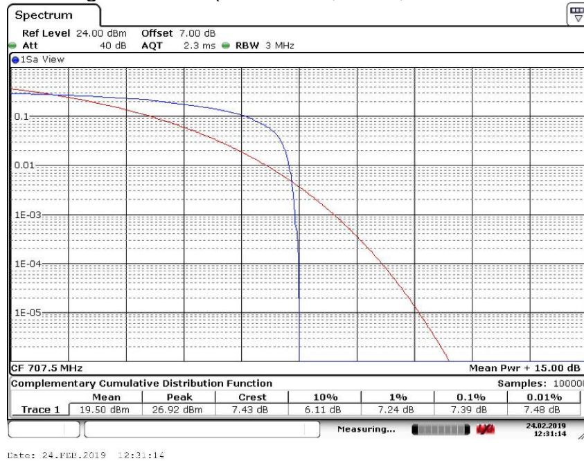
Peak-Average Ratio Plot(10MHz BW,QPSK,Band 12-mid Channel)
