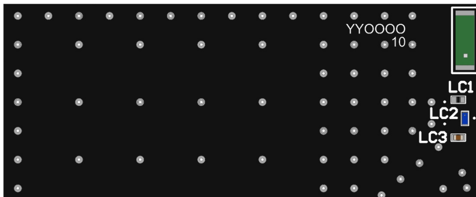
3D View of matching components and recommended values (LC1 = 0.3pF, LC2=1.0nH, LC3= 0.3pF)
