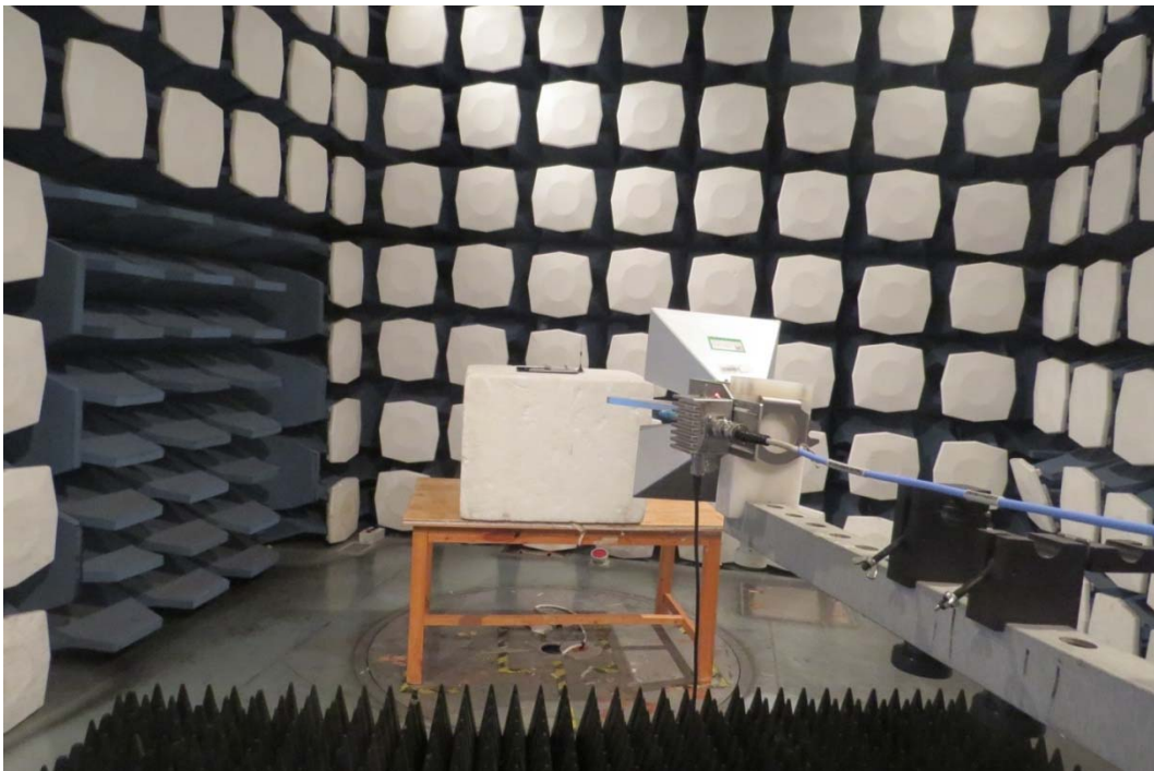
Picture 1: Radiated Spurious Emissions Test setup
